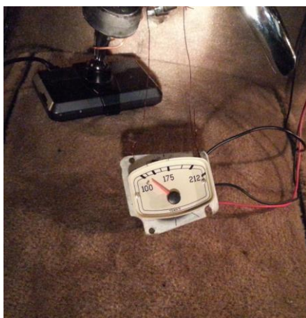
Switching on from cold: needle moves to low reading
